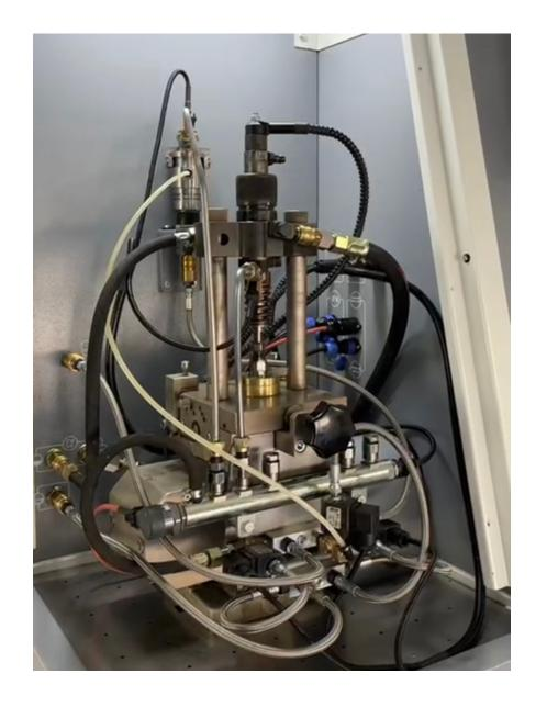
UTS1004 can test the Injector Delivery and Return flow of the F2e Non-Pumping Injector.
